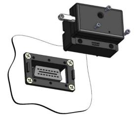
• Plug in the lock and fix it with the provided M3 screws
